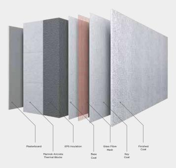
SIMS by Mannok combines the benefits of each building element to work together effectively in a way that is superior to the alternative methods. The key construction elements are:
